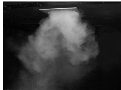
Flow development with vertical setting (only models 600/625)
