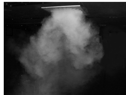
Flow development with vertical setting
